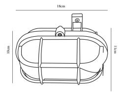
Voltage (V): 230 Volt IP degree if the fixture includes two types of IP degree: IP44 Maximum compatible bulb wattage (W): 60W Class (Class I, Class II, Class III): Class 2 (Double isolated) Lampholder type (eg, E27/E14, etc): E27 Parallel connection possible?: True
