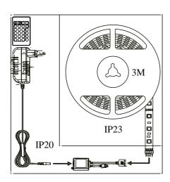
Voltage (V): 12 Volt IP degree if the fixture includes two types of IP degree: IP23 Class (Class I, Class II, Class III): Class 3 (12V) Lampholder type (eg, E27/E14, etc): LED Module
