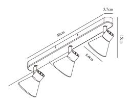
Voltage (V): 230 Volt IP degree if the fixture includes two types of IP degree: IP20 Maximum compatible bulb wattage (W): 35W Class (Class I, Class II, Class III): Class 1 (Earth contact) Lampholder type (eg, E27/E14, etc): GU10 Dimmerable: Yes with compatible bulb
