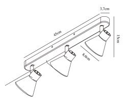
Voltage (V): 230 Volt IP degree if the fixture includes two types of IP degree: IP20 Maximum compatible bulb wattage (W): 35W Class (Class I, Class II, Class III): Class 1 (Earth contact) Lampholder type (eg, E27/E14, etc): GU10 Dimmerable: Yes with compatible bulb
