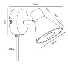
Voltage (V): 230 Volt IP degree if the fixture includes two types of IP degree: IP20 Maximum compatible bulb wattage (W): 35W Class (Class I, Class III): Class 2 (Double isolated) Lampholder type (eg, E27/E14, etc): GU10 Dimmerable: Yes with compatible
