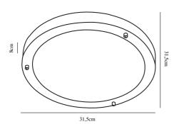
Voltage (V): 230 Volt IP degree if the fixture includes two types of IP degree: IP44/43 Maximum compatible bulb wattage (W): 2X40W Class (Class I, Class II, Class III): Class 1 (Earth contact) Lampholder type (eg, E27/E14, etc): E27
