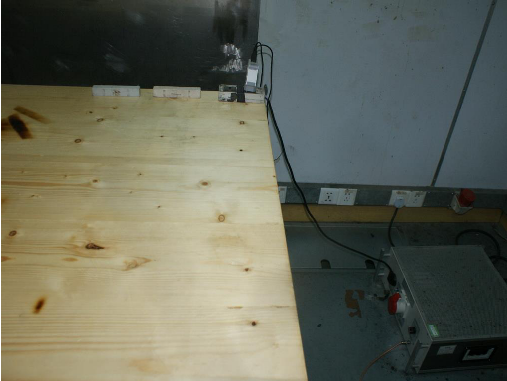
Photograph 2: Set-up for Radiated Disturbance (30-1000MHz)
