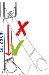
**GB** Slowly pull it down parallel to the wall. Grip the adhesive nail (adhesive screw) tightly when removing the strip.
