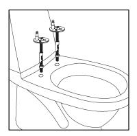
Assemble the bolts and hinges and insert them into the mounting holes in the toilet
