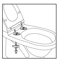
Position the locking bolt correctly Click the seat onto the hinges Close the seat and adjust to desired position, then open and remove the seat
