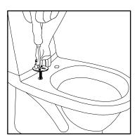
Lift up the hinge base and tighten the screws loosely with a screwdriver
