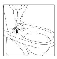
Lift up the hinge base and tighten the screws loosely with a screwdriver
