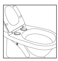
Tighten the bolts firmly and make sure the nut is positioned correctly Remove the seat and place the cove cap on the hinge base and press in place Click the seat back into place
