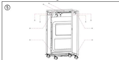
Put the (f) back panel on two side panels after you place the gas cylinder on the bottom plate. (Refer to Figure 6)
