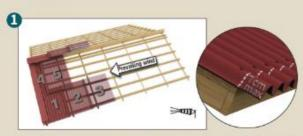
Laying in staggered rows avoids the superposition of 4 sheet thicknesses at overlap points. Always start your first row at the gutter, leaving maximum 7 cm overhang.
