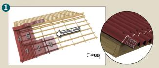
Laying in staggered rows avoids the superposition of 4 sheet thicknesses at overlap points. Always start your first row at the gutter, leaving maximum 7 cm overhang.
