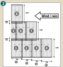
Sheets must be fixed onto each of their supporting battens. Every corrugation should be nailed at eaves, overlaps and ridges. Every second corrugation has to be fixed at the intermediate purlins. The fixing at the intermediate purlins has to be staggered.
