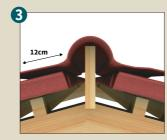
Use a ridge batten to support the Onduline ridge piece as shown. The ridge element has to overlap the ONDULINE® sheet min. 12 cm.
