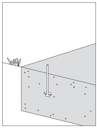
Place bolt and one washer in wet cement. Let cement harden.
