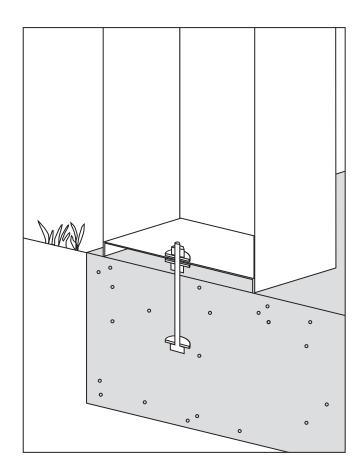
After some time, mount the mailbox in the middle hole in the bottom of the box with washer and nut.
