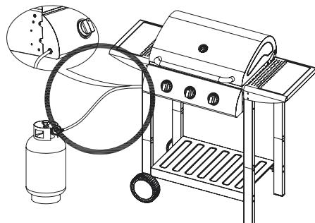
The gas bottle must be changed outside at a safe distance from naked flames and other sources of ignition.
