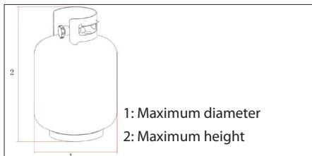
The maximum diameter and the maximum height of the gas bottle is 310 mm and 500 mm respectively, as indicated below.
