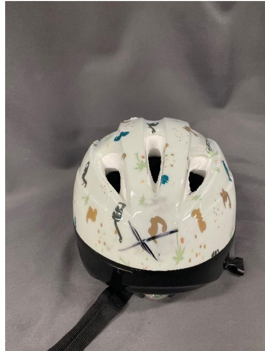
Picture 42. Impact point Helmet 1 44702. Back Flat.
