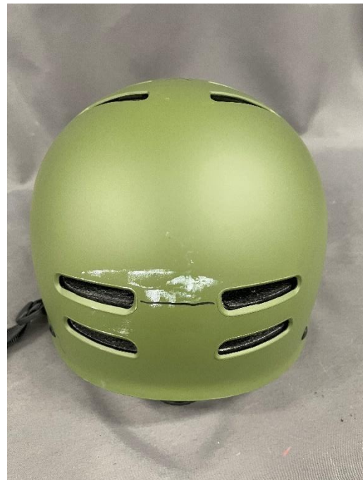
Picture 8. Impact point Helmet 2 44690. Back Kerb.
