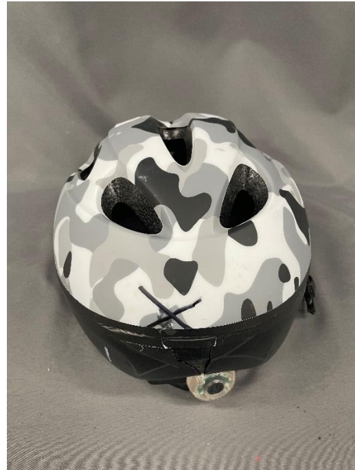
Picture 26. Impact point Helmet 1 44698. Back Flat.
