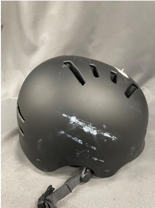
Picture 19. Impact point Helmet 3 44695. Side Kerbstone.
