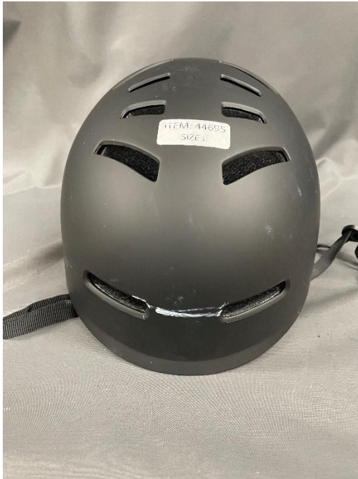
Picture 15. Impact point Helmet 1 44695. Front Kerbstone.
