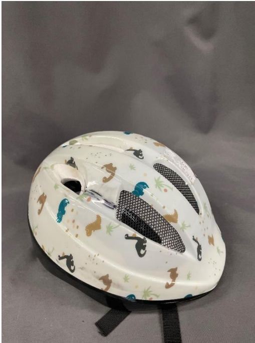
Picture 41. Impact point Helmet 1 44702. Crown Side Kerbstone.
