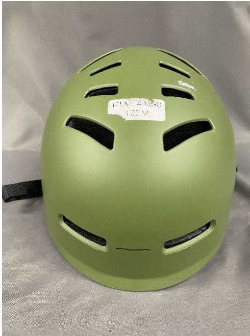
Picture 9. Impact point Helmet 3 44690. Front Kerbstone.
