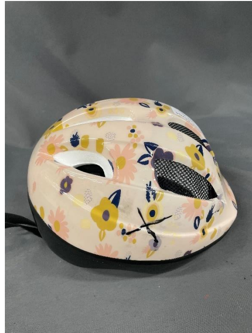
Picture 48. Impact point Helmet 1 44704. Side Flat.
