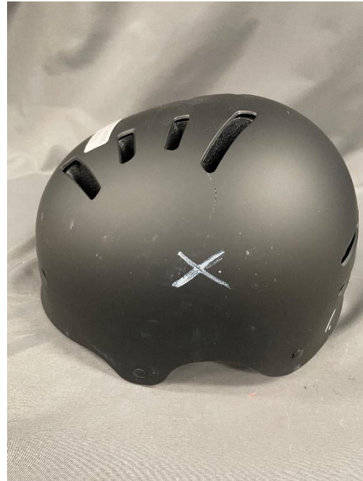
Picture 16. Impact point Helmet 1 44695. Side Flat.
