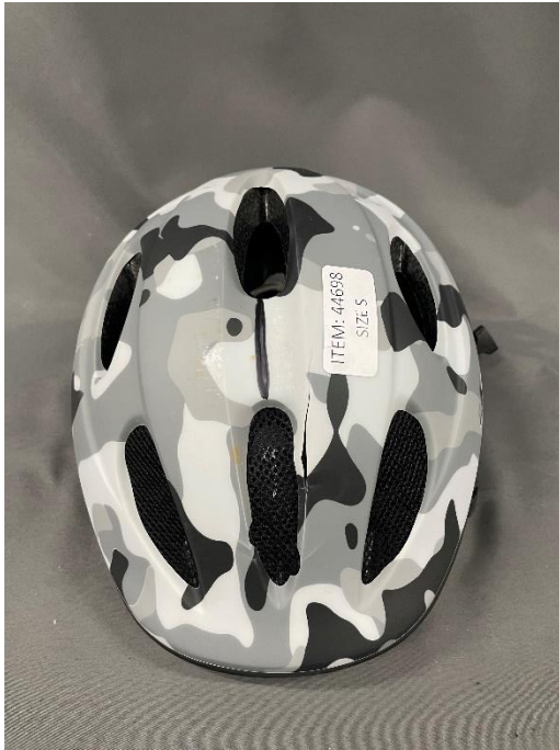
Picture 25. Impact point Helmet 1 44698. Crown Kerbstone.
