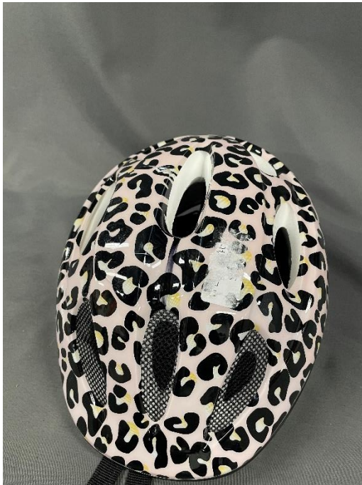
Picture 35. Impact point Helmet 2 44699. Crown Kerbstone.
