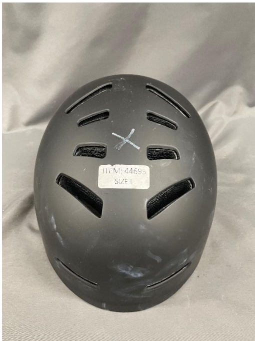
Picture 17. Impact point Helmet 2 44695. Crown Flat.
