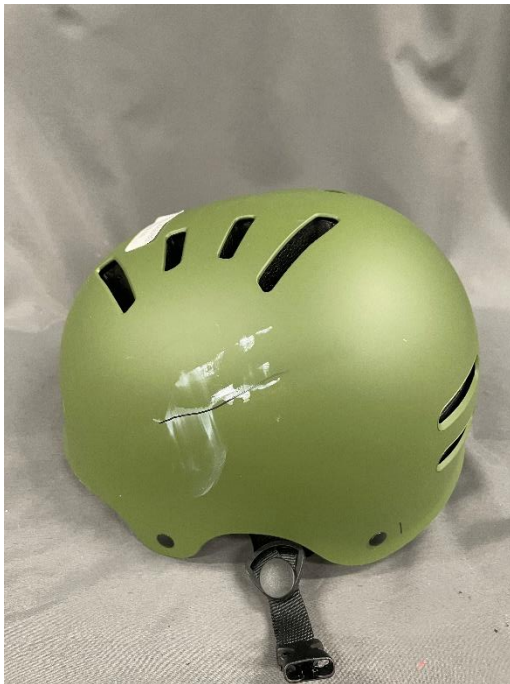
Picture 5. Impact point Helmet 1 44690. Side Kerbstone.
