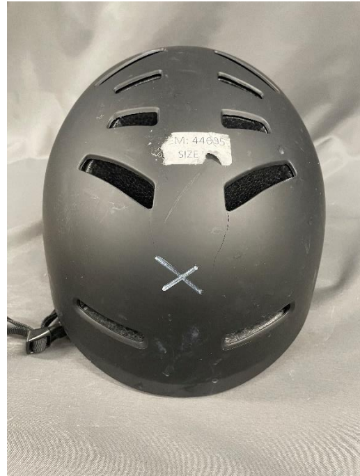
Picture 20. Impact point Helmet 3 44695. Front Flat.
