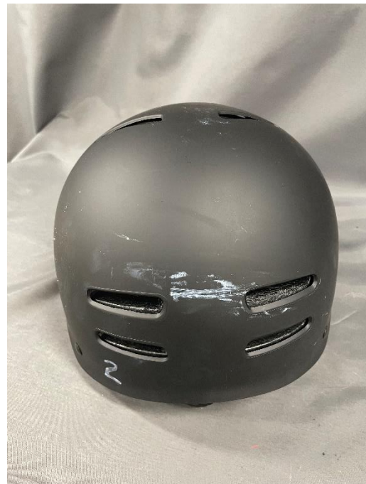
Picture 18. Impact point Helmet 2 44695. Rear Kerbstone.
